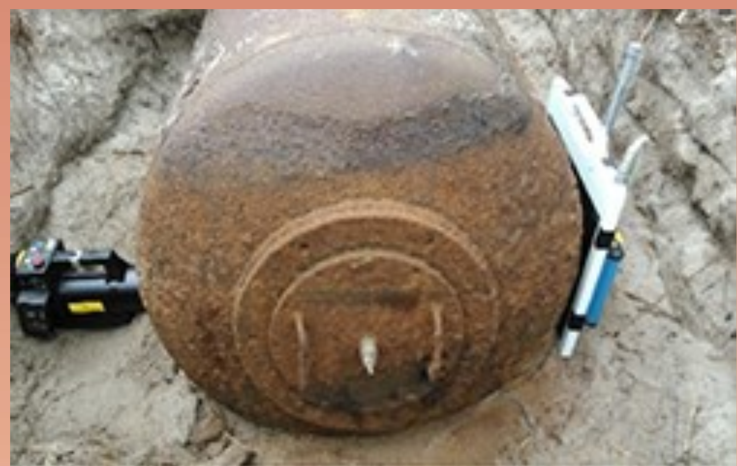
Figure 3: Xraying the M2 mine on site at Cape Henlopen. Photo courtesy of Jim Hall of Delaware State Park.
